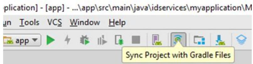
**Note:** To remove a dependency package, just delete the corresponding “*compile ...*” line in the *build.gradle* file and synchronize again the project.
